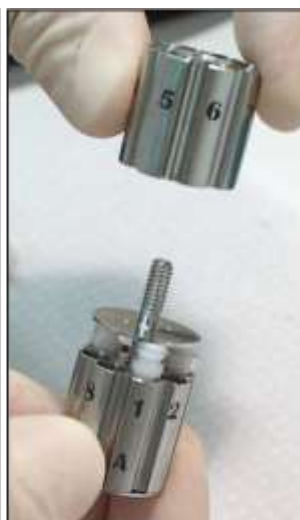
Insert connector piece into first cartridge.
