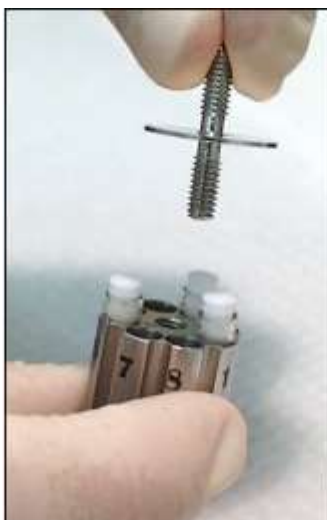
Place sample tubes into cartridge. Space samples evenly.
