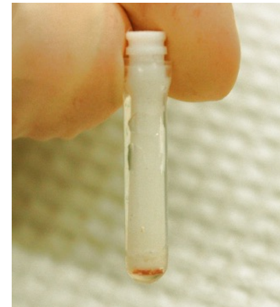
Insert MicroPestle using capper tool
